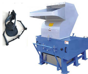
Plastic Crusher ---To crush and recycle the waste the material and defective goods
