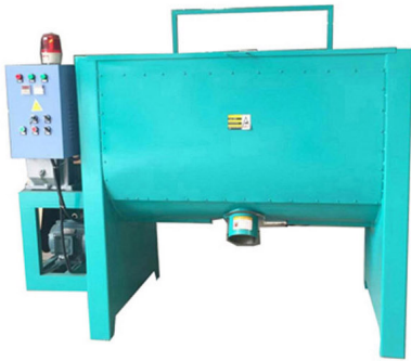
Dry Mixer ----To mix PVC resin powder and DOP softning oil
