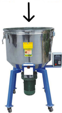
Color Mixer ---To mix pigment and other chemicals with mixed PVC and DOP material
